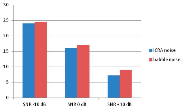
Using Comfort Digisystem in a situation with a SNR of -10 dB, the SNR was improved by up to 24 dB; the improvement in a situation where speech and noise level were equal, SNR 0, the improvement was up to 17 dB, and in +10 dB SNR, the improvement was up to 8 dB.
