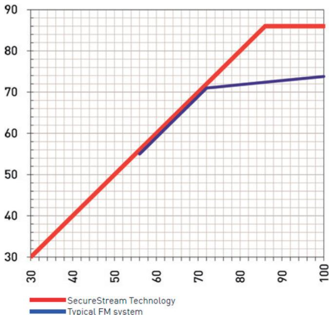
The graph indicates how weak and loud the transmitted signals can be. If there is insufficient dynamic range in any part of the transmission chain, the loud parts of speech are distorted while the weak sounds of speech will be masked by background noise. This means that speech perception is impaired.
